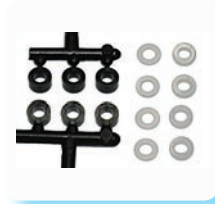
6466 Shock Downstop, (travel limiter), 4 ea. of 3 sizes 1/8" (.125"), 1/16" (.062") and 1/32" (.031")
