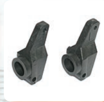
6366 Rear Hub Car- rier, 1.5° toe-in (per side). Requires special 3/16" X 3/8" flanged bearing #9277 (only fits #9275 or #7367 rear axles) B3
