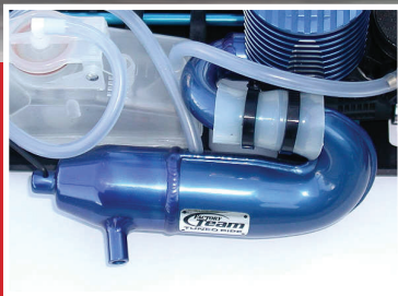
▶ Race-Proven Dual-Chamber Tuned Pipe
