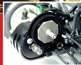
▶ High Torque Capacity Double-Sided Slipper
