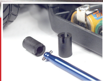
▶ 6061 T6 Blue Anodized Aluminum Drive Shaft
