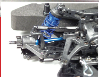
▶ Lightweight Foam Bumper and Threaded Aluminum Shock Bodies
