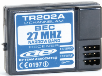
#29122 Receiver, TR202A 2 channels, 27AM. For NTC3, GT, B4, T4.
