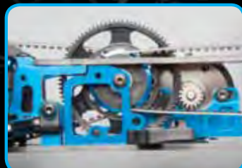
The spur gear has been lowered by 5mm achieving an overall lower center of gravity for the TC6 chassis
