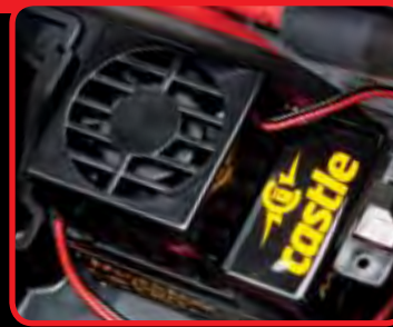
Mamba Max Pro electronic speed control with Deans® Ultra Plug® battery connector
