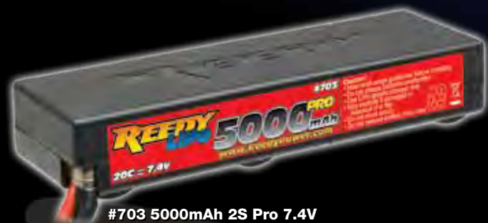
#703 5000mAh 2S Pro 7.4V Discharge: 20C (100A) continuous, 30C (150A) burst Weight: 293g Connector: None w/12 gauge wire + balance connector
