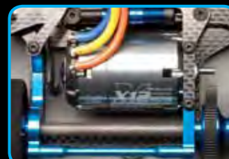
Updated wide rear pod allows easy installation of brushless motors and features machined aluminum motor mount, left bulkhead and standoff.
