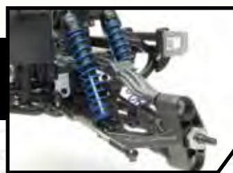
Eight oil-filled independent coil-over shock absorbers, 14.0mm steel drive hexes and heavy duty metal-gear hi-torque servo
