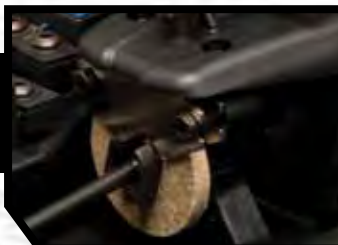
Independently adjustable front and rear disk brakes let you adjust the braking bias to suit your track conditions
