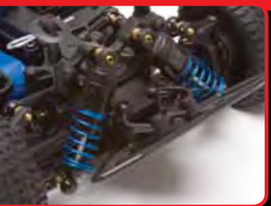
Composite shock with adjustable pre-load
