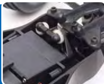
Angled "coplanar" steering with integral servo saver
