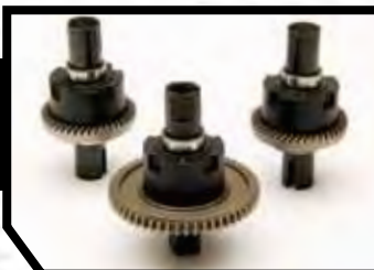
Factory assembled gear differentials come filled with specific silicone fluids, and are tuned for maximum performance.
