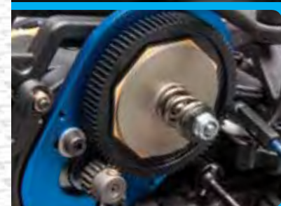
V2 slipper clutch with high-rate spring for consistent performance
