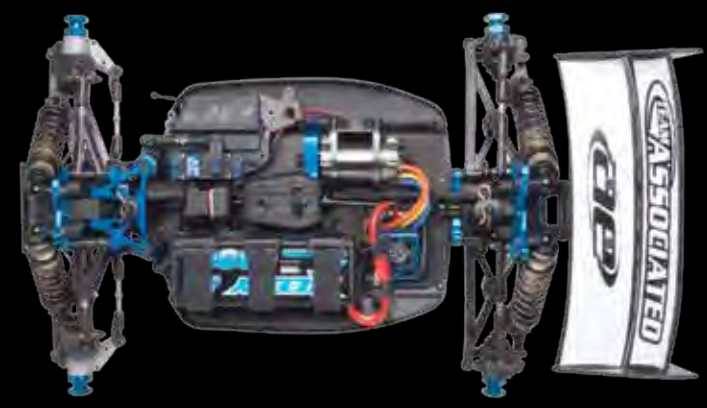
Pre-assembled Factory Team 16mm 'Big-Bore' threaded, hard-anodized shocks come ready to fill out of the box
