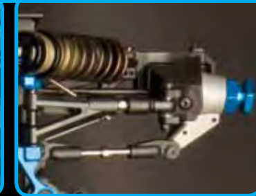
Updated steering geometry for more consistency through the rough and reduced bump-steer
