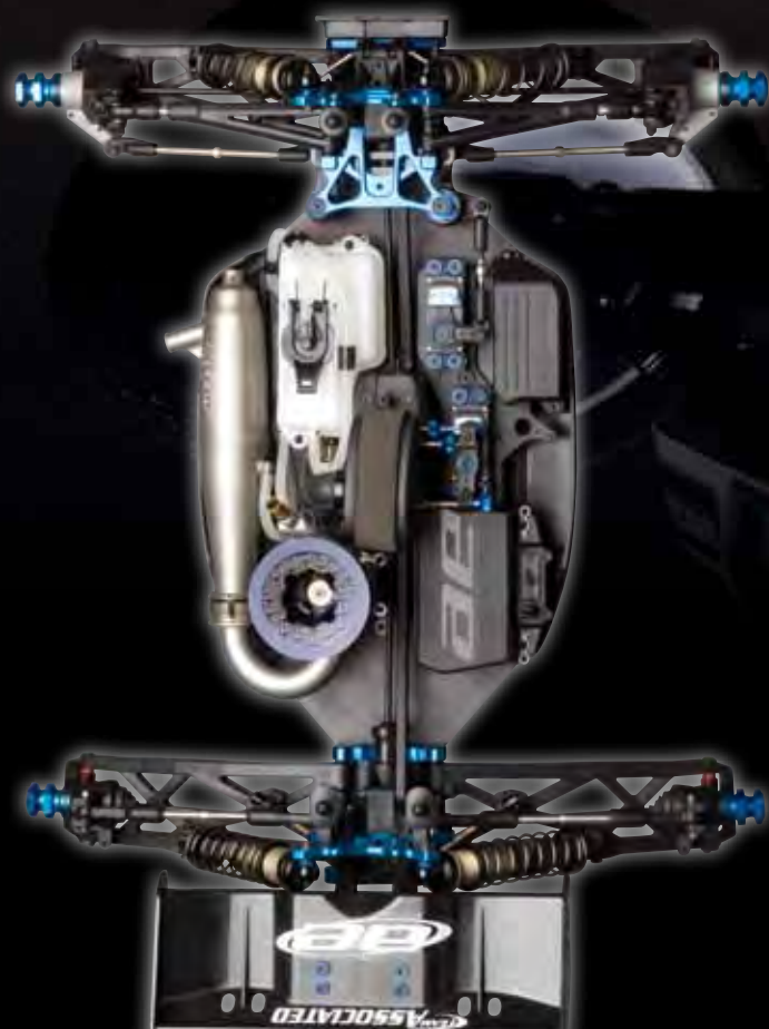
Factory Team machined blue aluminum top plate for superior strength
