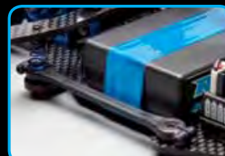
Factory Team pivot ball-link chassis allows for independent adjustment for roll, bump, and alignment. Accepts single cell LiPo batteries.
