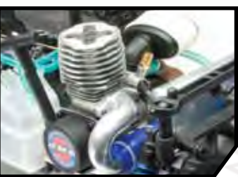
Team Associated AE-18 two-stroke nitro engine with pull-start with tuned exhaust and header pipe
