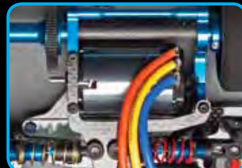
3-point upper pod plate is more open, allowing easier access and installation of brushless motors
