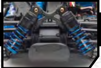
Fluid filled composite shocks
