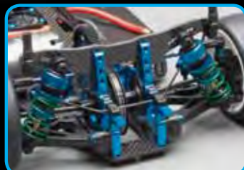
Adjustable differential height and belt tension titanium turnbuckles with ballcup eyelets aluminum clamping wheel hexes
