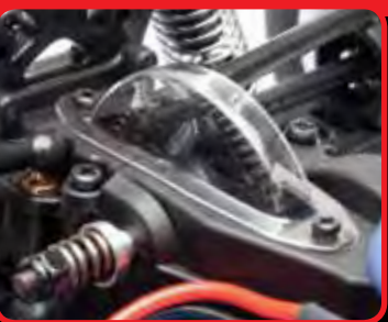
Sealed two-belt drive train
