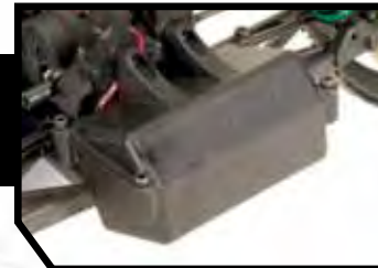
Sealed battery box keeps the receiver battery safe and secure
