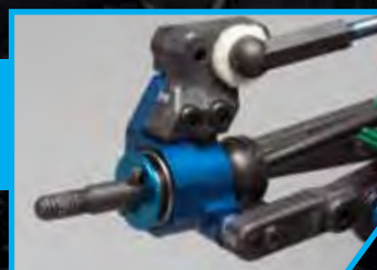
Factory Team 0.5 degree aluminum rear hubs with oversize outer bearing
