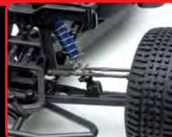
Rugged steel turnbuckles and blue aluminum shock bodies
