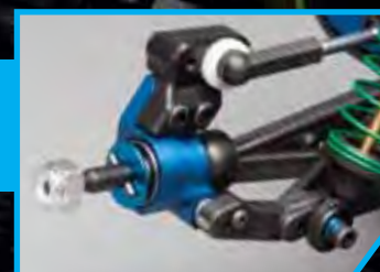
Factory Team 0.5 degree aluminum rear hubs with oversize outer bearing
