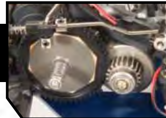
New more efficient dual-disc slipper clutch and large ball bearing clutchbell
