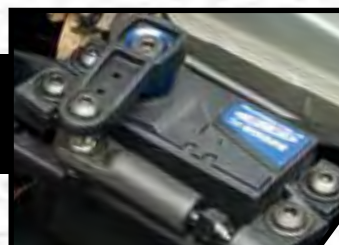
Precision S2008 Metal Gear steering servo and S1903 throttle servo features high-torque and high-speed
