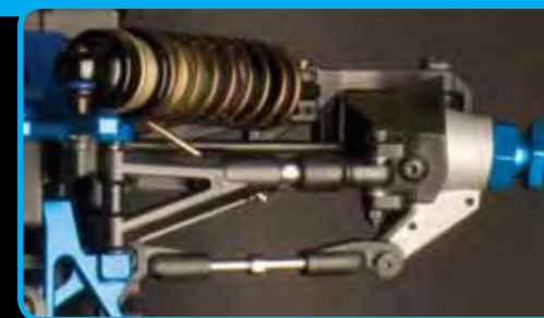
Updated steering geometry for more consistency through the rough and reduced bump-steer
