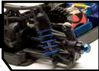
Silicone filled shocks
