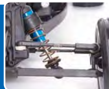
Tunable suspension with rugged steel turnbuckles
