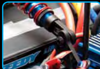
The Factory Team pivot ball-link chassis allows for independent adjustment for roll, bump, and alignment. 2.5mm woven carbon fiber chassis
