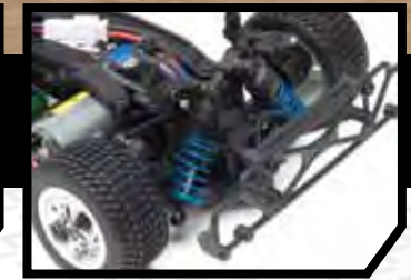
Composite shock with adjustable pre-load
