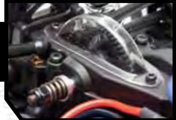
Sealed two-belt drive train with adjustable slipper clutch
