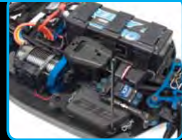
Receiver box, servo, and battery tray remove from car in one piece for easy cleaning
