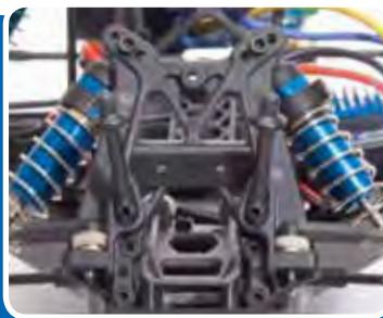
Fluid filled blue aluminum shock bodies front & rear
