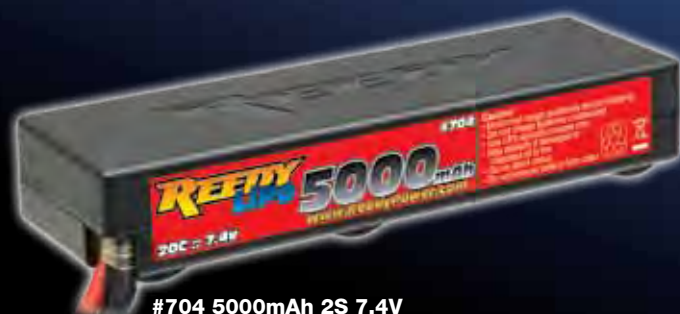
#704 5000mAh 2S 7.4V Discharge: 20C (100A) continuous, 30C (150A) burst Weight: 293g Connector: Tamiya style w/14 gauge wire + balance connector
