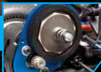
V2 slipper clutch with high-rate spring for finer adjustment increments
