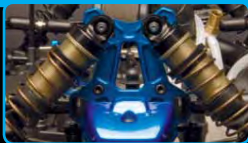
Updated 5mm 7075 blue aluminum shock towers and optimized upper camber link bushings
