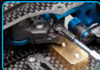
Updated steering system featuring more Ackermann options for improved steering input rate resulting in more consistent handling
