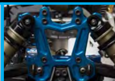
5mm machined blue aluminum shock towers for light weight strength, and durability
