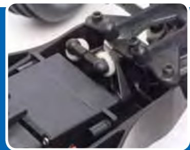
Angled "coplanar" steering with integral servo saver
