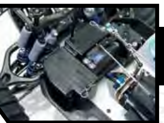
Sealed radio box and battery box
