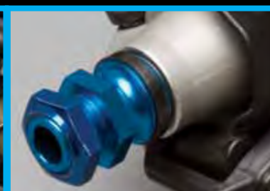
Blue aluminum narrow hex adapters with pin retainer clips and nylon locking wheel nuts
