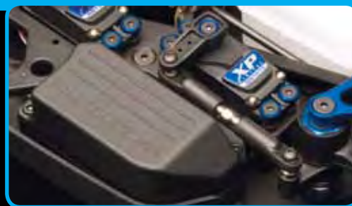
Molded composite radio tray with optional forward placement battery box for increased steering
