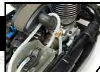
Team Associated 2-chamber muffler and header pipe are designed to work with .28 Pro engine to provide maximum power
