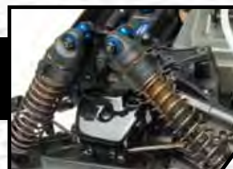
3mm low-profile black aluminum shock towers and installed anti-roll bars, front and rear
