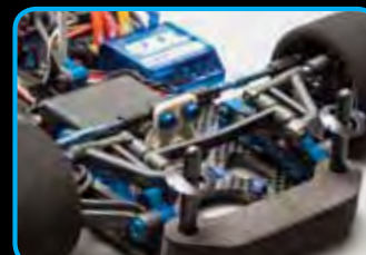
Active strut front end features symmetric components with adjustable caster and track width, as well as a new front axle with wheel nut.
