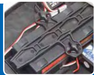
Battery strap with twist-lock thumb knobs for easy access
