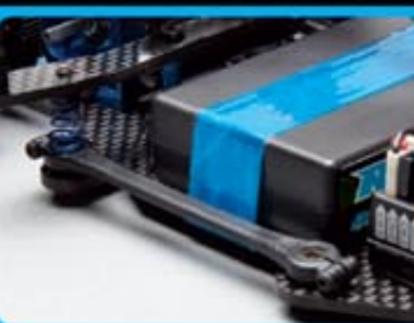
Factory Team pivot ball-link chassis allows for independent adjustment for roll, bump, and alignment. Accepts single cell LiPo batteries.
