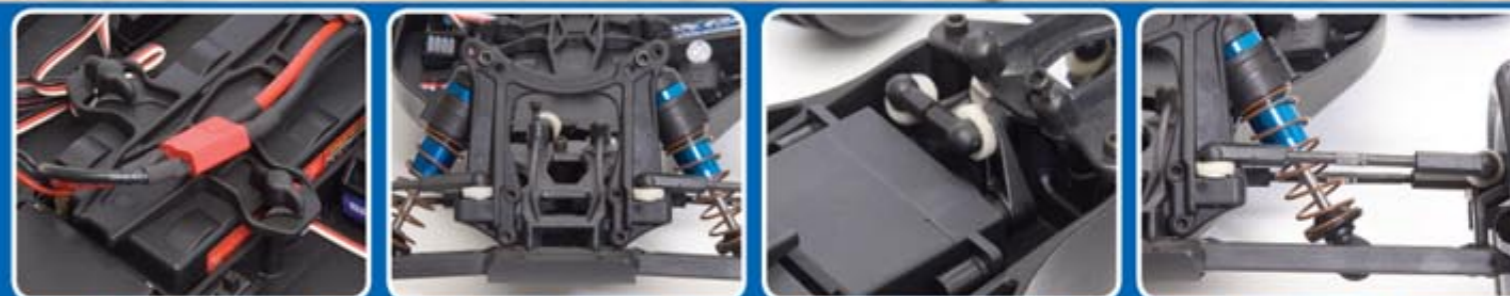
Battery strap with twist-lock thumb knobs for easy access
