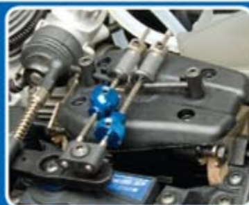
Sealed radio box with thread-through molded antenna mount keeps the receiver and batteries securely protected
