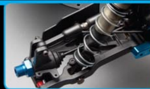
Factory Team 7075 blue aluminum steering knuckles with Factory Team aluminum axles, front and rear
