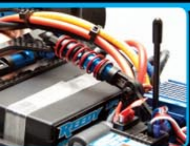
Factory Team shocks with through-shaft design making for equal damping in both directions. Woven carbon fiber center shock tower
