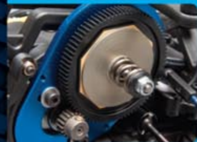
V2 slipper clutch with high-rate spring for consistent performance
