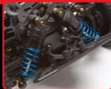
Composite shock with adjustable pre-load
