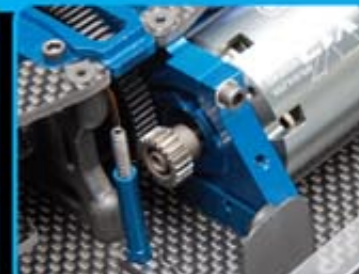
Factory Team blue aluminum cam motor mount set and V2 slipper clutch
