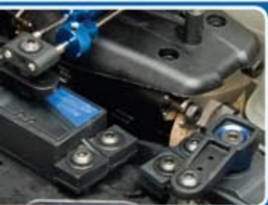
Precision S2008 Metal Gear steering servo and S1903 throttle servo features high-torque and high-speed
