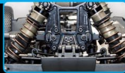
Factory Team 5mm 7075 aluminum low-center of gravity shock towers with optimized geometry
