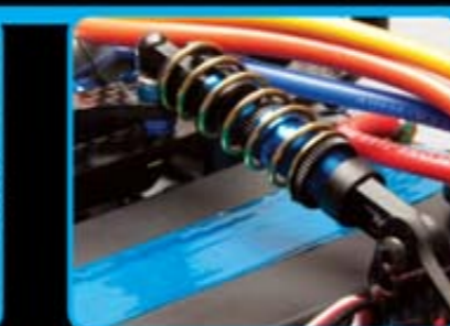
Factory Team shocks with through-shaft design making for equal damping in both directions. Woven carbon fiber center shock tower
