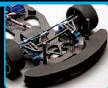
Updated active strut front end features symmetric components with adjustable caster and track width, as well as a new front axle with wheel nut.
