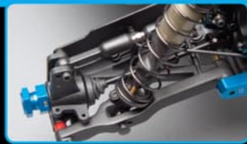
Newly designed suspension arms feature centerline shock mounts and optimized anti-roll bar position
