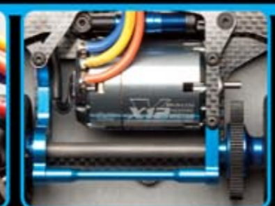
Updated wide rear pod allows easy installation of brushless motors and features machined aluminum motor mount, left bulkhead and standoff.
