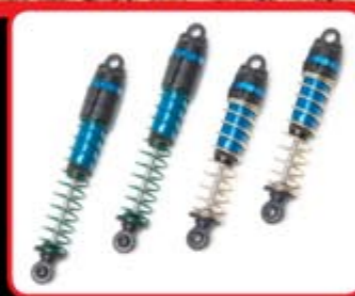
Blue anodized aluminum V2 coil-over shocks
