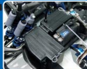
Sealed radio box and battery box
