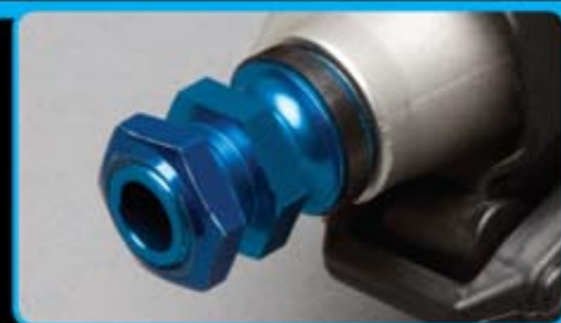
Blue aluminum narrow hex adapters with pin retainer clips and nylon locking wheel nuts
