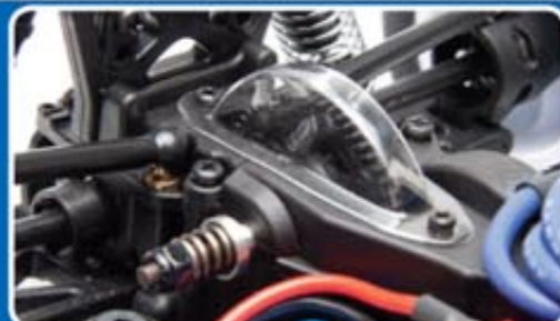
Sealed two-belt drive train with adjustable slipper clutch
