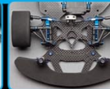
Woven carbon fiber front arm mounting plate makes for a stiffer front end assembly featuring indexed wheelbase options
