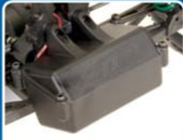
Sealed battery box keeps the receiver battery safe and secure
