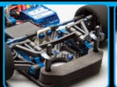
Active strut front end features symmetric components with adjustable caster and track width, as well as a new front axle with wheel nut.
