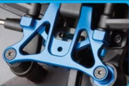
Factory Team machined blue aluminum top plate for superior strength
