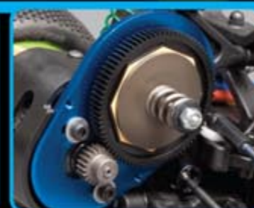
V2 slipper clutch with high-rate spring for finer adjustment increments
