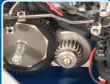
New more efficient dual-disc slipper clutch and large ball bearing clutchbell
