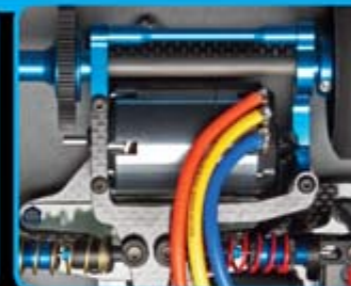
3-point upper pod plate is more span, allowing easier access and installation of brushless motors
