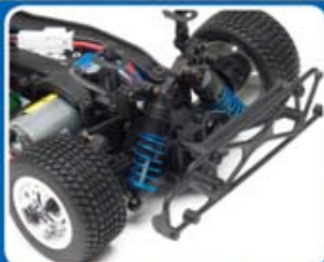
Composite shock with adjustable pre-load
