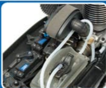
Team Associated 2-chamber muffler and header pipe are designed to work with .28 Pro engine to provide maximum power
