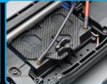
Centralized-mass battery mount with carbon fiber strap
