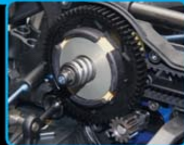
VTS4 slipper (variable torque, multi-plate slipper with four drive surfaces)
