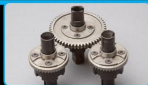
RC8T differentials come preassembled and ready to fill with diff fluid
