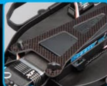
Carbon fiber battery strap
