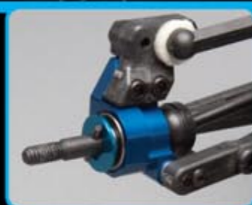
Factory Team 0.5 degree aluminum rear hubs with oversize outer bearing
