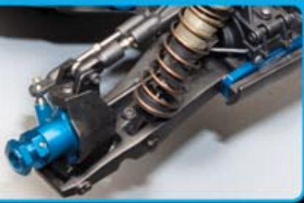
Factory Team 7075 blue aluminum steering knuckles with Factory Team aluminum axles, front and rear
