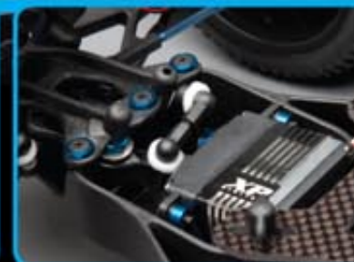
Angled bellcrank "coplanar" steering with integral servo saver
