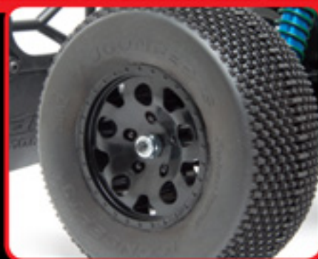
JConcepts rear tires and inserts on KMC® replica wheels
