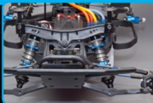
"Gull-wing" front suspension arms & updated shock towers optimized for 12mm big bore shocks
