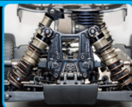
Factory Team 5mm 7075 aluminum low-center of gravity shock towers with optimized geometry
