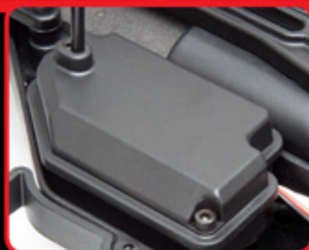
Water-Resistant enclosed receiver box
