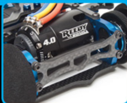
Optimized 3-point upper pod plate with graphite motor mount cross-brace
