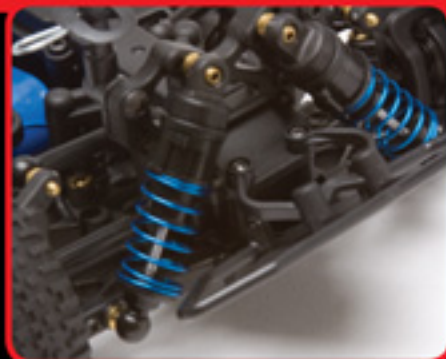
Composite shock with adjustable pre-load
