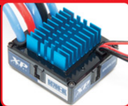
Water-Resistant XP SC700 with Deans® Ultra Plug® battery connector
