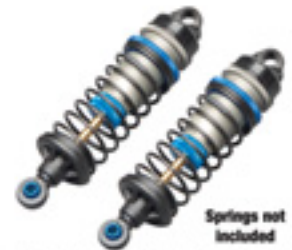
#91314 12MM Big Bore Shock Kit (Front) B4-B44
