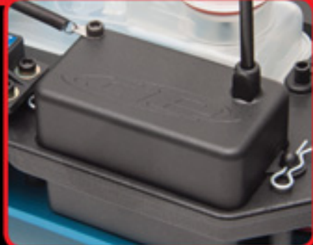
Water-resistant enclosed receiver box and battery box
