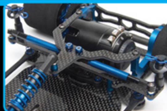
Side damper tubes, updated rear pod links and a 2.5mm thick chassis
