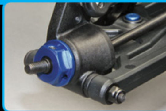
Factory Team machined blue aluminum wheel hex adapters
