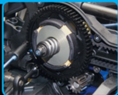
VTS4 slipper (variable torque, multi-plate slipper with four drive surfaces)
