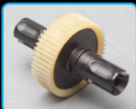
Ball differential with Factory Team light-weight outrives
