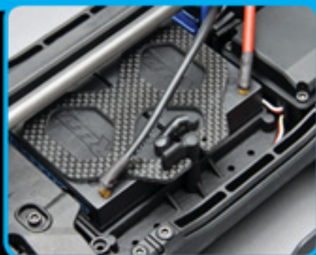
Centralized-mass battery mount with carbon fiber strap
