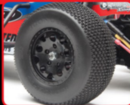
High traction rear racing tires on KMC® replica hex-drive wheels
