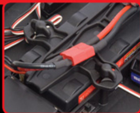
Battery strap with twist-lock thumb knobs for easy access
