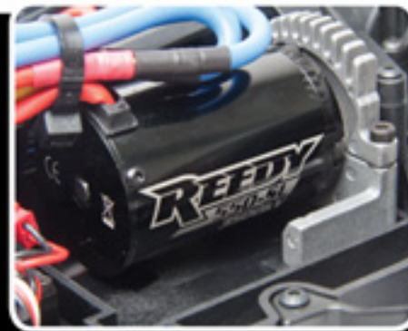
Brushless Reedy 550-SL 3500kV motor
