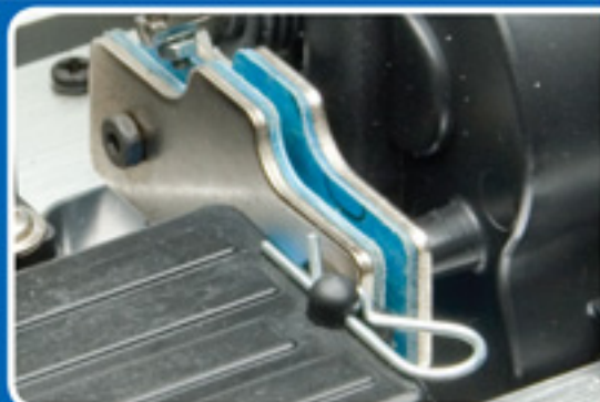
Massive braking power provided by the disk brake slows down the MGT8.0 quickly
