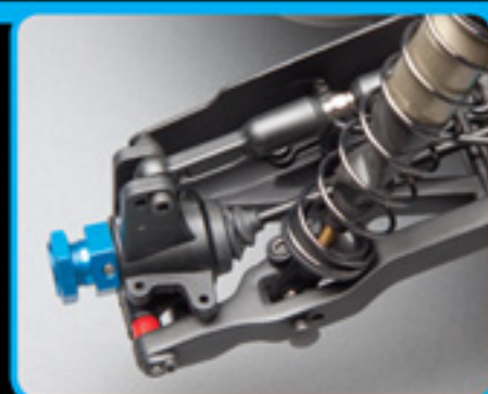
Newly designed suspension arms feature centerline shock mounts and optimized anti-roll bar position
