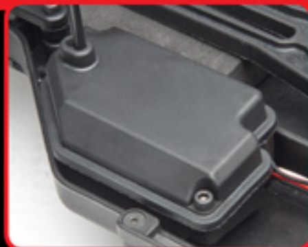
Water-Resistant enclosed receiver box
