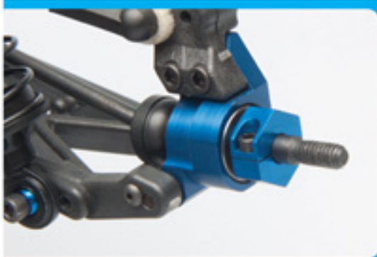
Factory Team 0° aluminum rear hubs with 12mm clamping hexes
