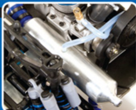
High-performance tuned exhaust pipe with single outlet
