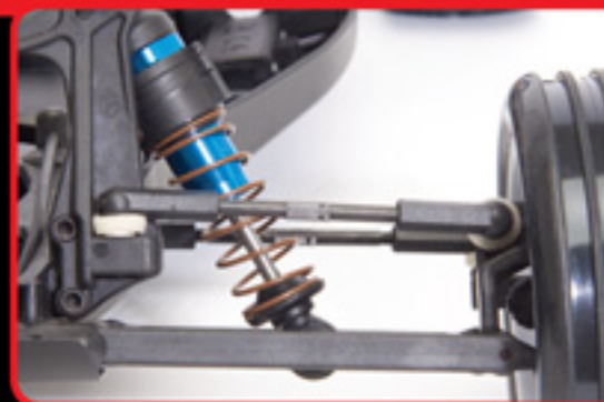
Tunable suspension with rugged steel turnbuckles
