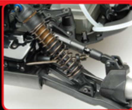
3mm low-profile black aluminum shock towers and installed anti-roll bars, front and rear
