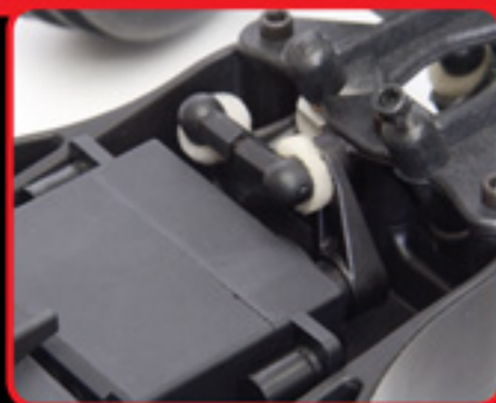
Angled "coplanar" steering with integral servo saver
