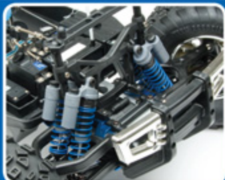
Eight oil-filled independent coil-over shock absorbers, and heavy duty metal-gear hi-torque steering servo
