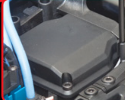
Enclosed water-resistant receiver box with removable ESC tray
