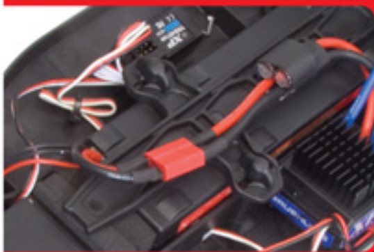
Battery strap with twist-lock thumb knobs for easy access
