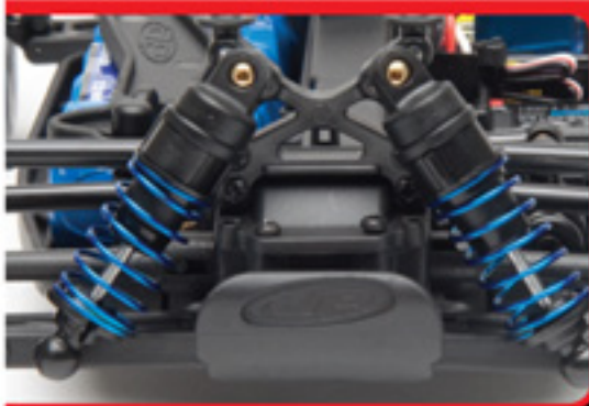
Fluid filled composite shocks
