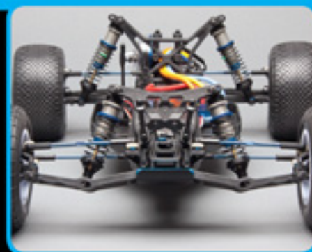
"Gull-wing" front suspension arms & updated shock towers optimized for 12mm big bore shocks
