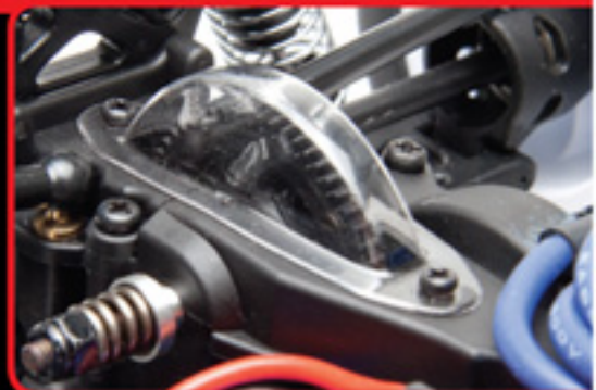
Sealed two-belt drive train
