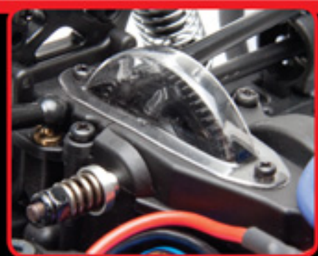
Sealed two-belt drive train with adjustable slipper clutch
