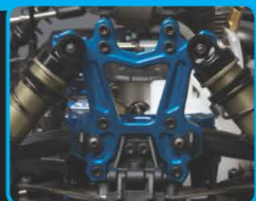
5mm machined blue aluminum shock towers for light weight strength, and durability
