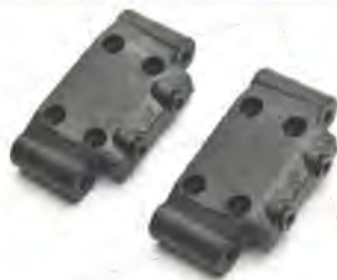
Adjustable front suspension mount angle 'kick-up' options of 25° and 30°
