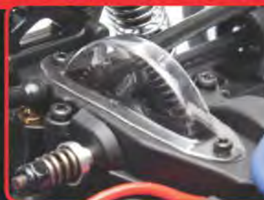
Sealed two-belt drive train
