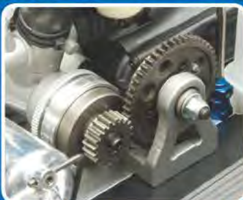
The 2-speed automatic transmission with reverse has improved durability to handle the massive power of the Team Associated 8.0 engine
