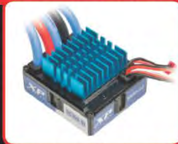
Water-Resistant XP SC700 with a high power battery connector
