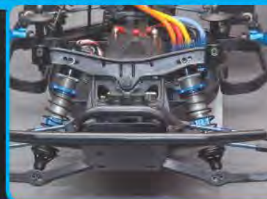
"Gull-wing" front suspension arms & updated shock towers optimized for 12mm big bore shocks
