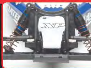
Fluid filled blue aluminum V2 shocks FT/RR Tunable suspension w/Rugged steel turnbuckles
