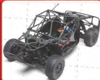
Functional full roll cage with integral dirt shields
