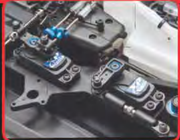
High torque XP DS1510MG metal gear steering servo
