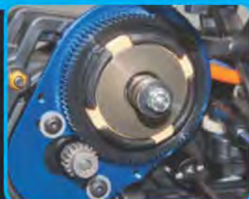
VTS slipper clutch with high-resolution spring for finer adjustment increments
