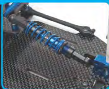
Innovative through-shaft center shock
