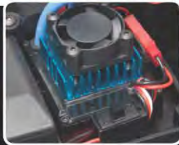
Water-Resistant XP SC900 with a high power battery connector
