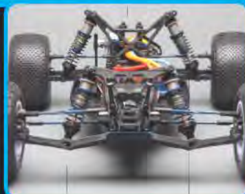
"Gull-wing" front suspension arms & updated shock towers optimized for 12mm big bore shocks
