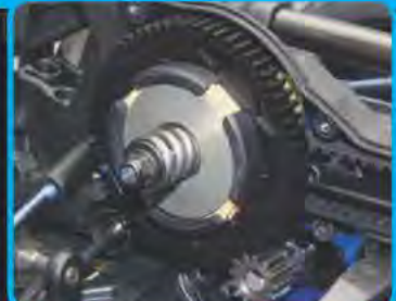
VTS4 slipper (variable torque, multi-plate slipper with four drive surfaces)
