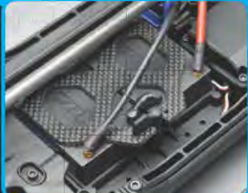
Centralized-mass battery mount with carbon fiber strap
