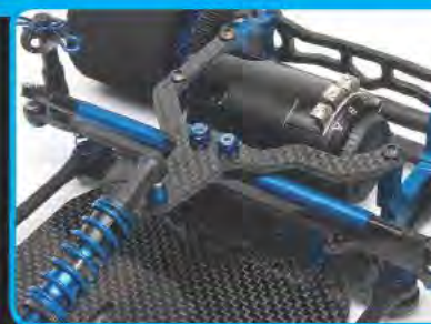
Side damper tubes, updated rear pod links and a 2.5mm thick chassis
