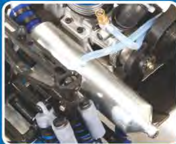
High-performance tuned exhaust pipe with single outlet
