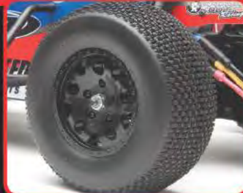
High traction rear racing tires on KMC® replica hex-drive wheels
