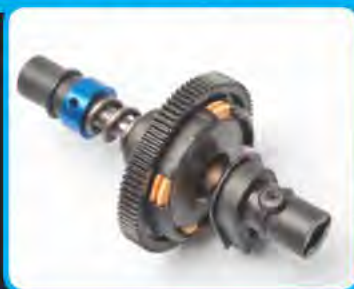
VTS slipper assembly with high-rate spring
