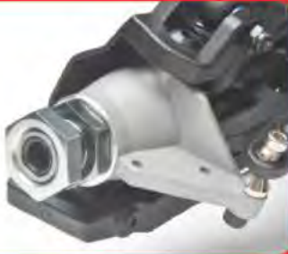
Aluminum steering knuckles for improved durability
