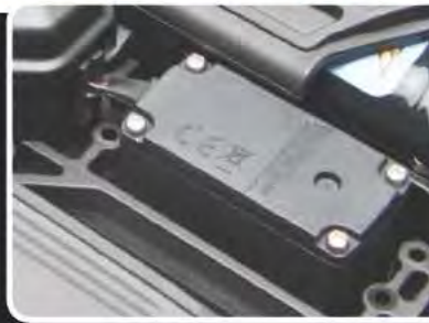
XP high torque metal gear servo
