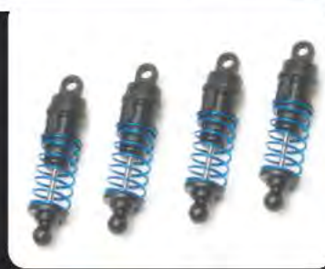
Adjustable fluid filled coil over shocks
