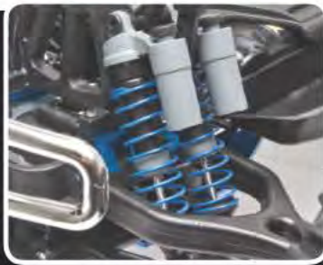
8 adjustable fluid filled coil-over shocks
