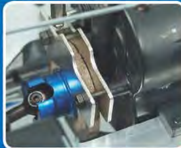
Large disc brake for positive, no-fade stopping power
