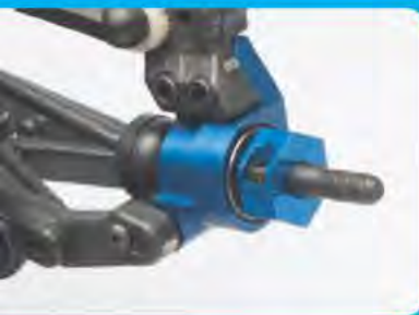
Factory Team 0° aluminum rear hubs with 12mm clamping hexes
