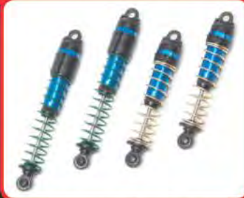
Blue anodized aluminum V2 coil-over shocks
