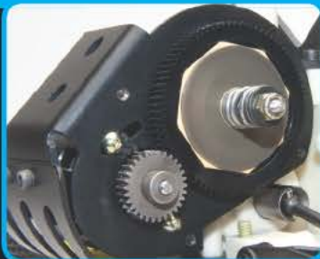
Stealth 3-gear transmission with ball differential and V2 slipper assembly
