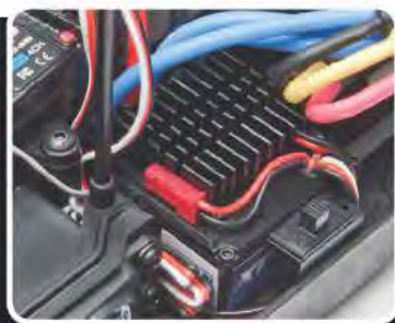
Water-Resistant XP speed control with a high power battery connector
