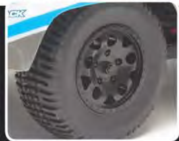
KMC® replica hex drive wheels mounted with aggressive short course racing tires
