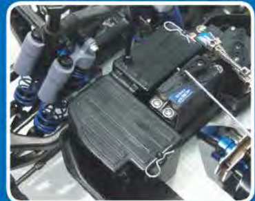
Sealed receiver box protects radio gear from the elements
