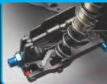
Factory Team 7075 blue aluminum steering knuckles with Factory Team aluminum axles, front and rear
