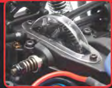
Sealed two-belt drive train with adjustable slipper clutch
