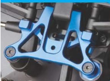
Factory Team machined blue aluminum top plate for superior strength
