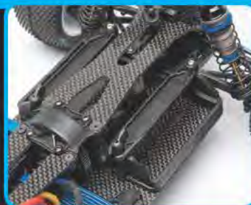
Composite battery trays with integrated spacers and quick change battery straps
