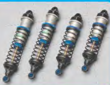
Factory Team 12mm 'Big Bore' hard anodized aluminum threaded shocks
