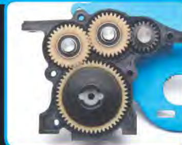
New transmission has stronger gears and a 14 carbide ball differential
