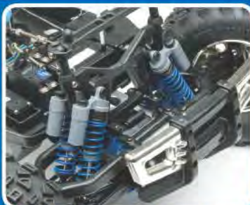
Eight off-filled independent coil-over shock absorbers, and heavy duty metal-gear hi-torque steering servo
