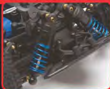
Composite shock with adjustable pre-load
