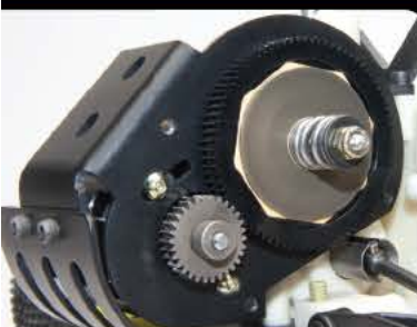
Stealth 3-gear transmission with ball differential and V2 slipper assembly
