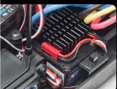
Water-resistant XP brushless electronic speed control
