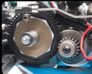
V2 dual disc slipper clutch with low center of gravity transmission
