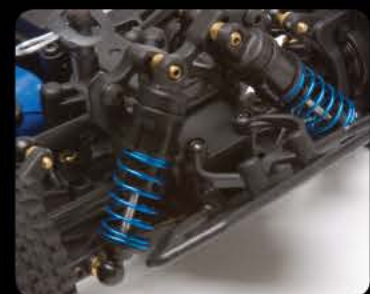
Composite shock with adjustable pre-load
