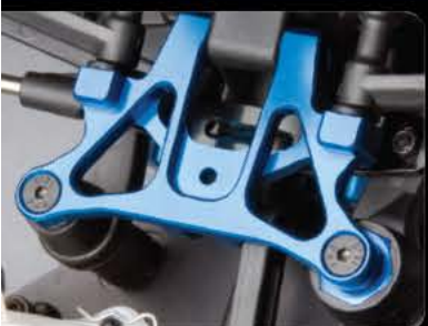
Factory Team machined blue aluminum top plate for superior strength
