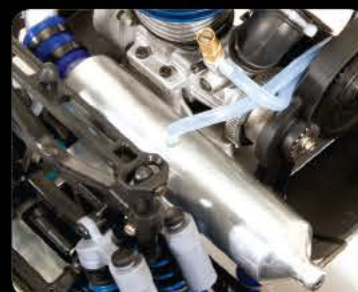
High-performance tuned exhaust pipe with single outlet
