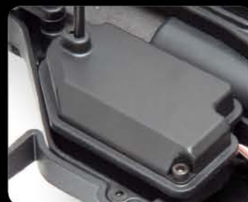
Water-resistant enclosed receiver box
