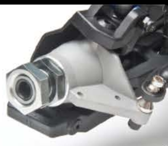
Aluminum steering knuckles for improved durability
