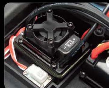
Splash-proof Reedy brushless speed control with High Current T-plug Connector
