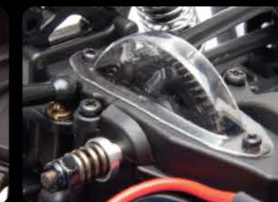
Sealed two-belt drive train
