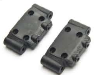
Adjustable front suspension mount angle 'kick-up' options of 25° and 30°
