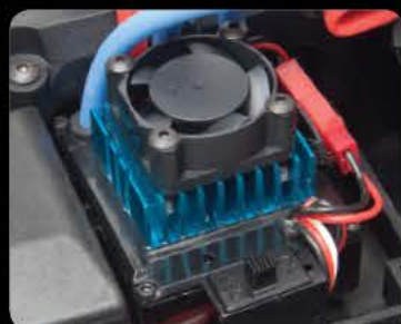
Water-Resistant XP speed control with High Current T-plug connector
