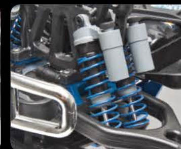
8 adjustable fluid filled coil-over shocks
