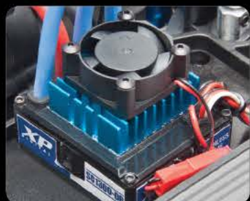
Water-resistant XP SC1300-DB brushless ESC with dual high power battery connector
