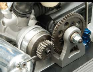
The 2-speed automatic transmission with reverse has improved durability to handle the massive power of the Team Associated 8.0 engine
