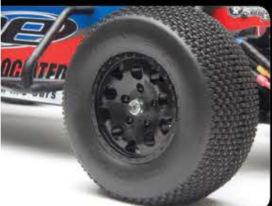
High traction rear racing tires on KMC® replica hex-drive wheels
