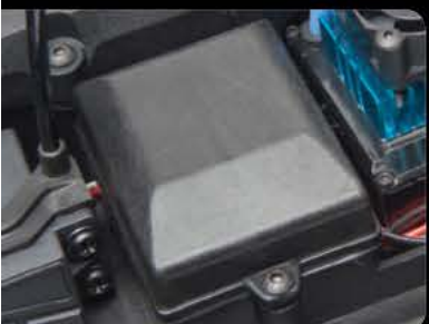
Water-Resistant enclosed receiver box
