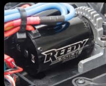
Brushless Reedy 550-SL 3500KV motor
