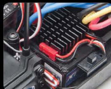
Water Resistant XP brushless electronic speed control
