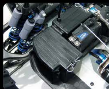
Sealed receiver box protects radio gear from the elements
