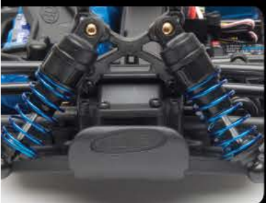
Fluid filled composite shocks
