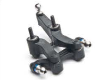
Updated steering system with horizontal ball studs for finer Ackermann adjustments
