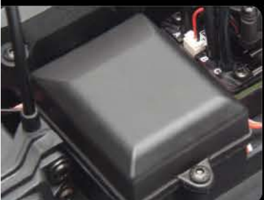
Water-resistant enclosed receiver box
