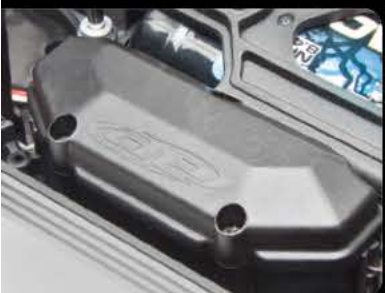
Water-resistant enclosed receiver box
