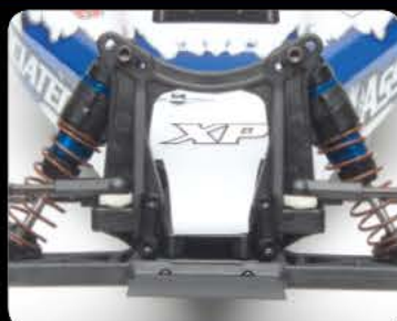
Fully tunable suspension with fluid filled blue aluminum V2 coil-over shocks
