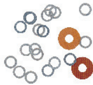
446 Shim Kit. Precision shims for spacing armatures. Five each of .010", .005", & .003" sizes. Comes with instructions. Will also fit any 1/8" shaft or pin for removing excess end play. (Not for 1:18 scale motors.)
