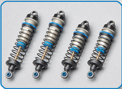
Factory Team 12mm "Big Bore" hard anodized aluminum threaded shocks
