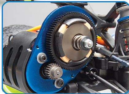
VTS slipper clutch with high-resolution spring for finer adjustment increments
