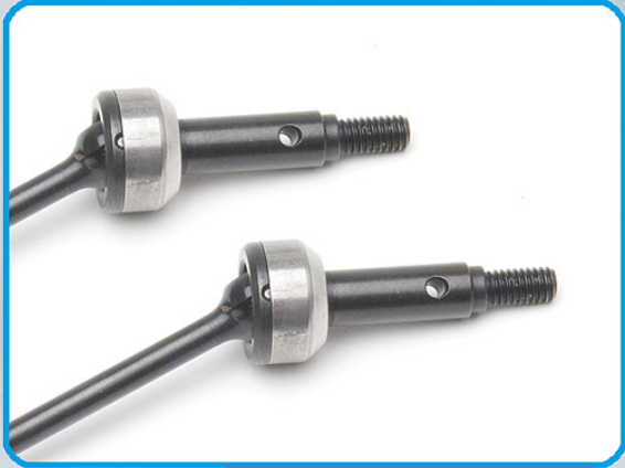
CVAs with captured drive pins and heavy duty 6mm alloy axles
