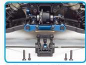
Gearboxes feature a 3.38:1 internal gear ratio with fast access differentials for quick removal, tuning and maintenance
