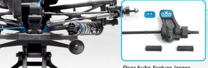
Rear hubs feature larger bearings and insert system to adjust camber link and rear toe-in
