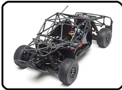
Functional full roll cage with integral dirt shields
