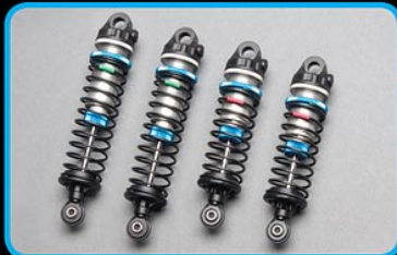
Factory Team V2 12mm "Big Bore" hard anodized aluminum shocks
