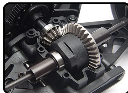
Front and rear sealed metal gear differentials and tough aluminum drive shaft
