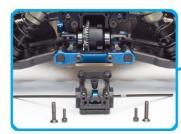
Gearboxes feature a 3.38:1 internal gear ratio with fast access differentials for quick removal, tuning & maintenance
