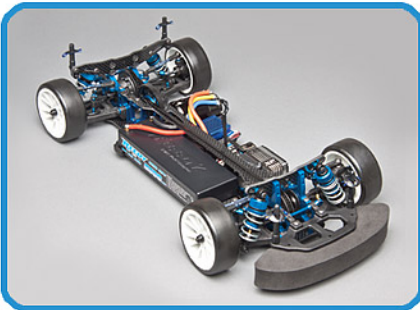
Ultra-narrow chassis layout optimized for LiPo batteries and brushless motors
