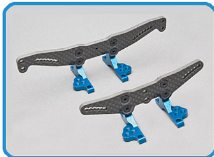
Factory Team vertical ballstud bearing caps with carbon-fiber shock towers
