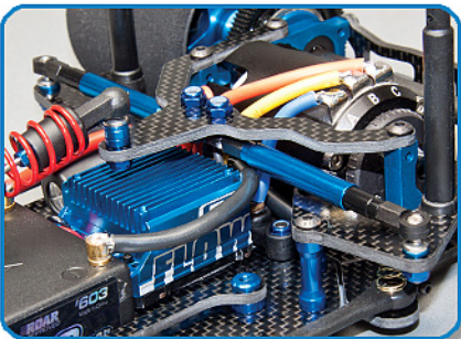
Side damper tubes reduces friction for smoother rear pod movement
