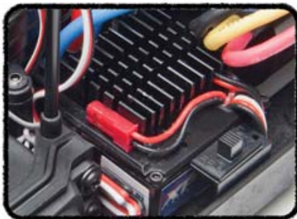
Water resistant XP brushless electronic speed control
