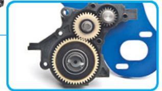
New transmission has stronger gears and a 14 carbide ball differential
