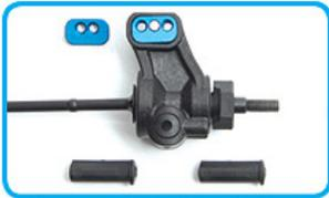
Rear hubs feature larger bearings and insert system to adjust camber link and rear toe-in
