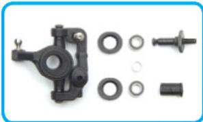
Steering and caster block insert system allows for easy caster and trailing axle adjustments
