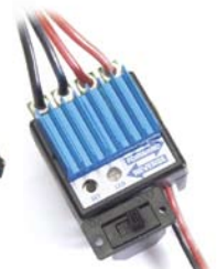
XPS speed control installed
