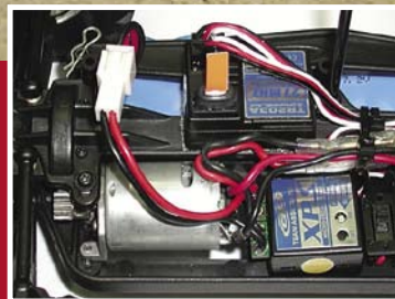
► Motor, Receiver, Speed Control, Servo, and Batteries Installed
