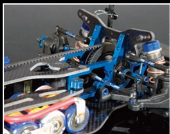
Newly designed composite ball differentials are super light for reduced rotational mass
