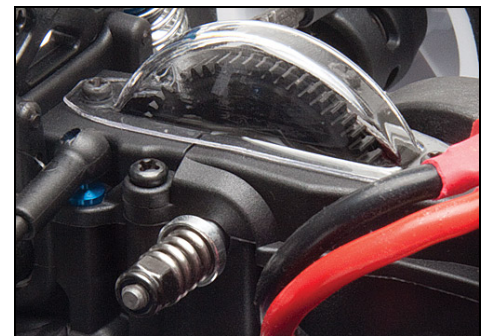
Sealed two-belt drive train with adjustable slipper clutch
