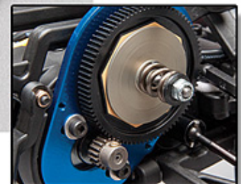
Below: V2 slipper assembly with high-rate spring and Factory Team Gold pads
