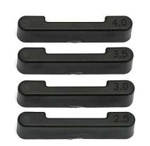
Includes new #7487 rear arm mounts that allow 4 choices of rear toe-in. This feature allows you to adjust the amount of rear toe-in to suit your track conditions.
