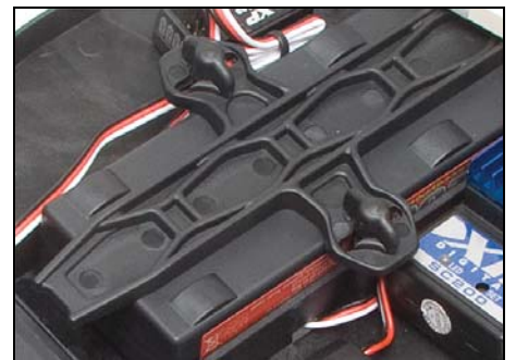
Battery strap with twist-lock thumb knobs.
