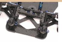
options package. We started with a **redesigned** graphite chassis, now flat-fronted with twin minibumpers for impact-damage resistance, and with tweak reference center
