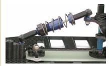
The rear suspension has also been optimized for 4-cell **competition**, using a single VCS Micro-Shock, a thicker, more
