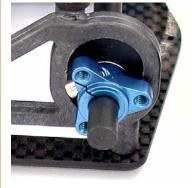
The blue 7075 T-6 aluminum rear hubs are all new, with a **single**clamp style left hub, and a dual-bearing supported right diff **hub** featuring the large
