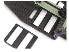
to file the graphite chassis battery cutouts. These trays provide approximately .150" (4mm) of battery movement to shift the weight of the cells forward for more steering, or backward for more rear traction.
