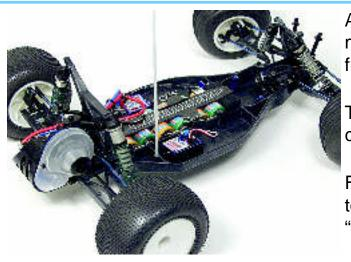
Angled bellcrank steering minimizes bump steer to maintain constant steering angles throughout the full range of suspension travel.
