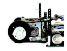
The rear chassis brace and T-bar have been redesigned and a T-bar brace was added. It also comes with a new precision lightweight left rear bulkhead for accurate bearing alignment. The redesigned upper and lower pod plates along with the left bulkhead make it easier to install, remove and solder in the motor.
