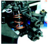
Pivot-ball type suspension with easily adjustable caster, camber, and toe-in. Interchangeable front and rear hub corners.
