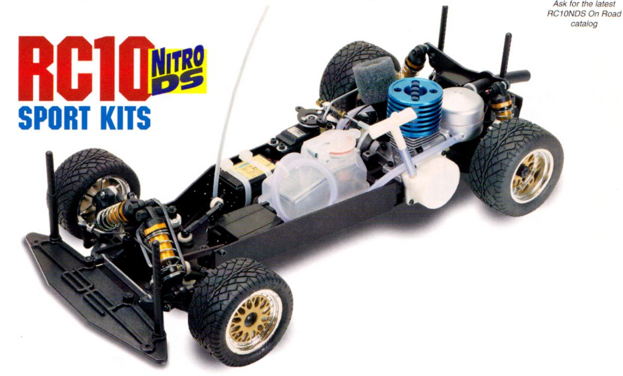
The RC10 Nitro DS Sport Kit differs from the Racer Kit in that it features bronze bushings instead of ball bearings, standard gold-anodized shocks, sport "Silencer" muffler, and mounting hardware for most .12 size pull start engine.
