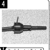
align holes. install pin all through axle and bone
