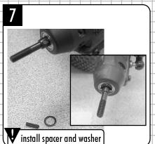
Re-install tire assembly on car. Continue building remaining CVD units and install on car.
