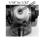
Idle Speed: 1/32" to 1/16" opening (.8 to 1.6mm) Larger opening = higher idle speed. Smaller opening = lower idle speed.
