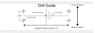
**Step 2** Drill the holes indicated on the drill guide: four 2.5mm holes and one 7mm hole. Once you are finished drilling, remove the drill guide.
