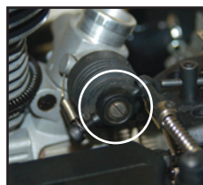
Low Speed Mixture: 6 1 / 4 turns out at full throttle Clockwise = Leaner Counterclockwise = Richer
