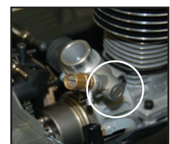
Mix Metering Screw: Even with carb body Clockwise = Leaner Counterclockwise = Richer
