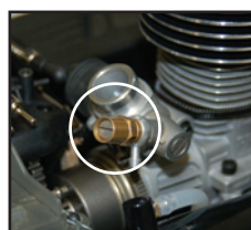
High Speed Mixture: 2 3 / 4 turns out Clockwise = Leaner Counterclockwise = Richer
