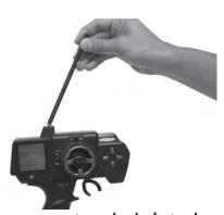
Screw antenna into the hole in the top of the transmitter.
