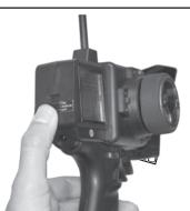
Move the switch on the transmitter to the ON position (blue LED will illuminate). Hold Transmitter with left hand ás shown.
