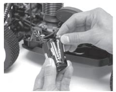
Insert 4 AA batteries (not included) or charged 5-cell NiMh pack into harness and install into radio box.
