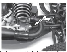
Slide the starter shaft though the back of your RC8T and into the hex starter on the back of the engine (body removed for clarification). Pull the trigger on the Pro Start to start engine.
