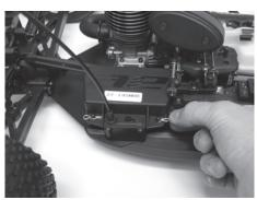
Use supplied clips to attach cover onto radio box.
