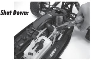
**CAUTION! Engine parts WILL be hot!** To shut your RC8T off, use pliers to pinch the fuel line, using **caution** to not rip the fuel line. Once engine is off, turn off your vehicle, then turn off your transmitter.
