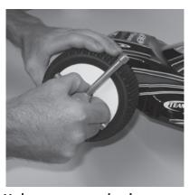
Make sure your wheel nuts are tight by holding the wheel, and tightening each wheel with the included wheel nut wrench.
