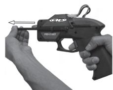
Remove starting bit from the holder on the side of the Pro Starter.
