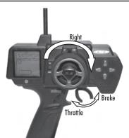
Check the operation of the radio system. Turn the steering wheel left and right. The front tires should turn left and right. Pull the trigger towards is set to neutral. See page 40 in your manual for setup instructions.
