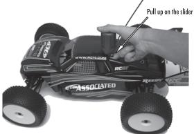
Insert the glow igniter into the remote glow plug. Make sure it 'grabs' the glow plug.
