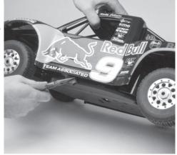
To shut your SC8 off, use pliers to pinch the exhaust deflector.
