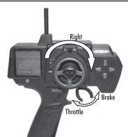
Check the operation of the radio system. Turn the steering wheel left and right. The front tires should turn left and right. Pull the trigger towards
