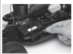
Use supplied clips to attach cover onto radio box.
