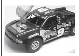
Attach body to chassis with the supplied body clips.
