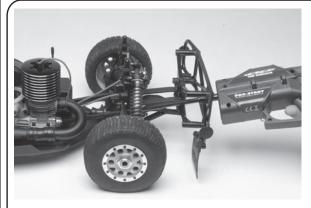
Slide the starter shaft though the back of your SC8 and into the hex starter on the back of the engine (body removed for clarification). Pull the trigger on the Pro Start to start engine.
