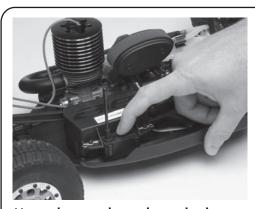
Move the switch on the radio box to the ON position.
