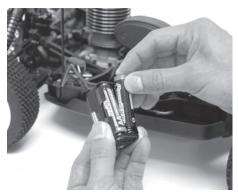
Insert 4 AA batteries (not included) or charged 5-cell NiMh pack into harness and install into radio box.
