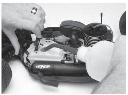
Lift the fuel tank lid and, using the supplied fuel bottle, fill the tank with fuel (not included).
