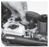
Prime the fuel tank by squeezing the primer bulb until fuel reaches the carbureator.
