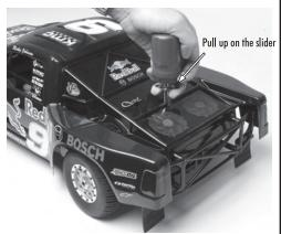
Insert the glow igniter into the remote glow plug. Make sure it 'grabs' the glow plug.
