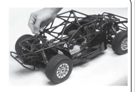
Attach roll cage to chassis with the supplied body clips.
