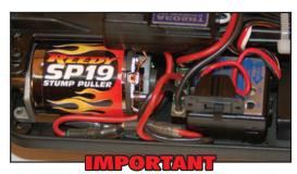
Because your new Reedy motor is slightly longer than the stock motor, you MUST move the Electronic Speed Control (ESC) forward and relocate the switch, as shown in the picture above. A piece of double-sided tape has been included to help you do that.
