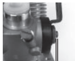
1/16" Low Speed Mixture: 1/16" of screw showing (1.5 mm)
