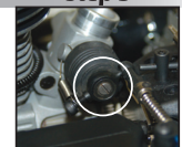
Low Speed Mixture: 4 1/2 turns out at full throttle Clockwise = Leaner Counterclockwise = Richer
