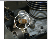
High Speed Mixture: 3 turns out Clockwise = Leaner Counterclockwise = Richer
