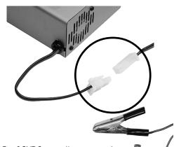
For 12VDC operation, connect the DC adapter cord's plug to the plug connected to the rear of the charger.
