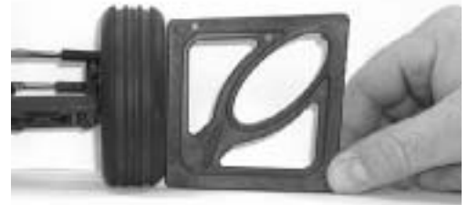
Testing camber with the camber gauge
