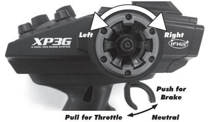
Throttle set to Neutral when turning on the radio!
