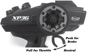
Throttle set to Neutral when turning on the radio!
