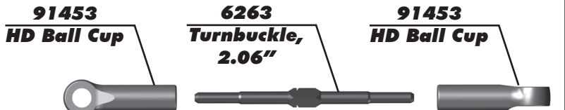
Rear Camber Turnbuckle 23.50mm
