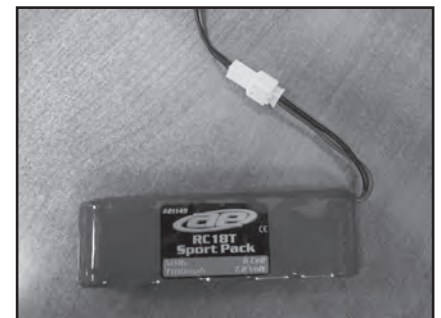
Plug wall charging jack into battery pack. (Battery must charge a full 10 hours.)
