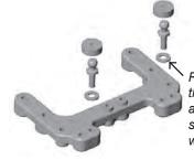
Raise or lower the ball end by adding or subtracting washers here
