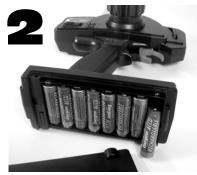
...(8 AA cells) as shown above. Be sure to use only high-quality alkaline or rechargeable Ni-Cd AAsize batteries.
