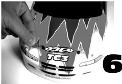
...securing it to the chassis with four body clips, two in the front, and two in the posts through the rear window Be sure to feed the antenna through the hole in the body.
