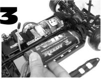
... by removing the battery brace, place the battery pack followed by the foam battery spacer, and resecuring the battery brace with the body clips.
