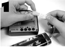
...by plugging it into your battery charger (not included) and following the manufacturer's recommended charging procedure. When it is fully charged, remove it from the charger and get ready to install it into your truck.
