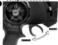
...following the speed control's instruction sheet. The speed control's one-touch setup system senses neutral, full throttle, and full reverse from your transmitter.
