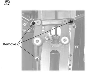
NOTE! Carefully remove servo saver from servo.
