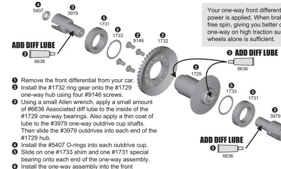
Your one-way front differential will turn the front wheels when power is applied. When braking, the front wheels will be allowed to free spin, giving you better cornering ability. We recommend the one-way on high traction surfaces where braking ability by the rear
